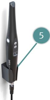
5. Place the camera in the camera holster to turn the camera off.
